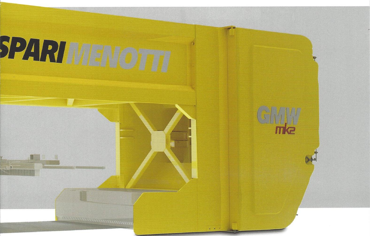
The sawing structure is made in a welded steel plate boxed structure designed to achieve maximum rigidity and minimum deformation. The diamond wire tensioning forces, both on the motor side and on the tensioning side, are symmetrically discharged by means of the shaft supports on the sawing structure which, thanks to its indeformability, guarantees no vibrations and the constant tensioning of the wires.
