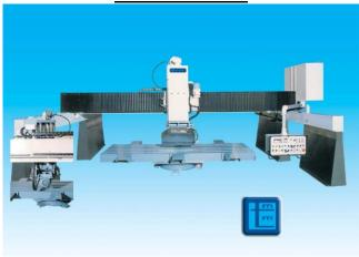
Machine designed for the cut of marble, granite and generic stones.
