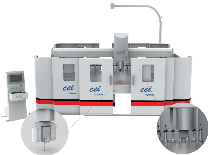
Tool storage up to 30 tools with automatic exchange
