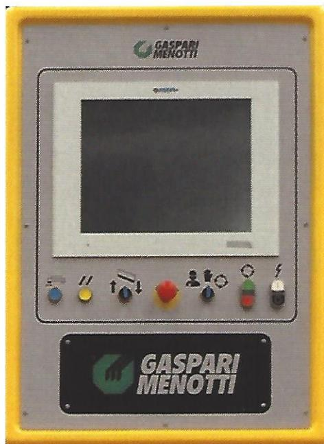
The new polishing machine is completely wired in FIELD BUS SYSTEM, with consequent simplification of the wiring, granting a reduction of faults possibility and, in case, a faster and timely search of these.
