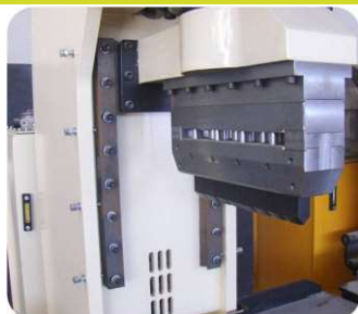
Cutting Head with Independent Blades (tools)
