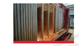
McLanahan's tailings management solutions dewater thickened solids resulting in a drip-free material that can be easily transported with mechanical handling equipment and potentially sold or used for land rehabilitation. These solutions not only make the waste material easier to handle, but also eliminate the need for settling ponds.
